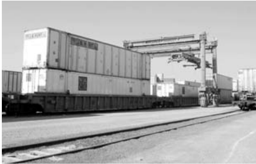
Class I railroads move much of their freight in containers, seen here being loaded in a major intermodal facility. Local transloading facilities can help smaller companies containerize shipments that otherwise would not move on the Class I system.
