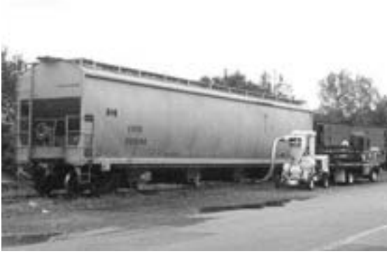
Transloading facilities may be as simple as the pumping unit seen next to this railcar. The pump transfers product to trucks for local delivery. The railcar holds the equivalent of four truck loads.
